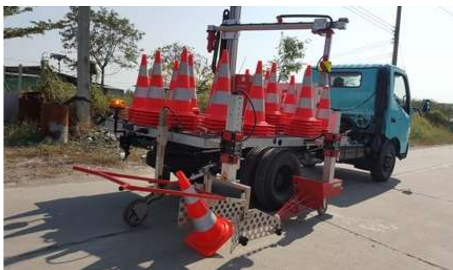
Figure 9. Example of Automated Cone Machine.
