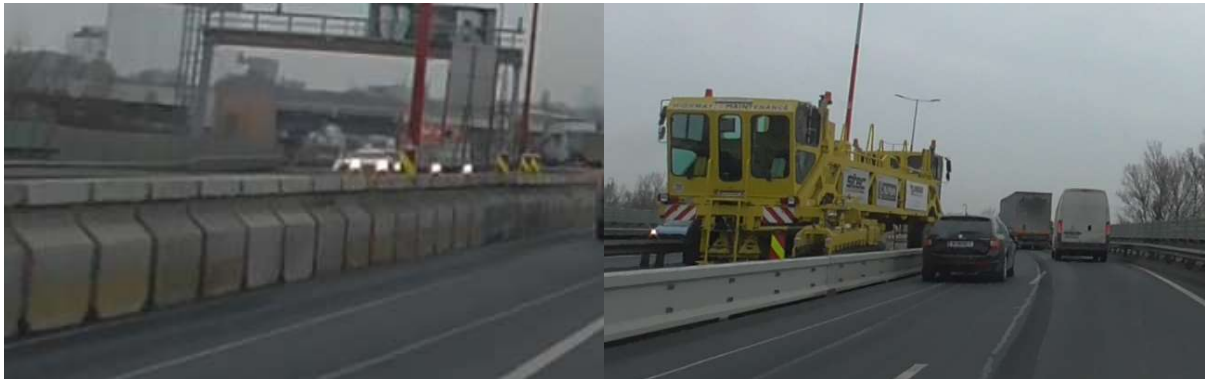
Figure 24. Quick moveable barrier and vehicle for application/moving of barriers. Source: KFV
