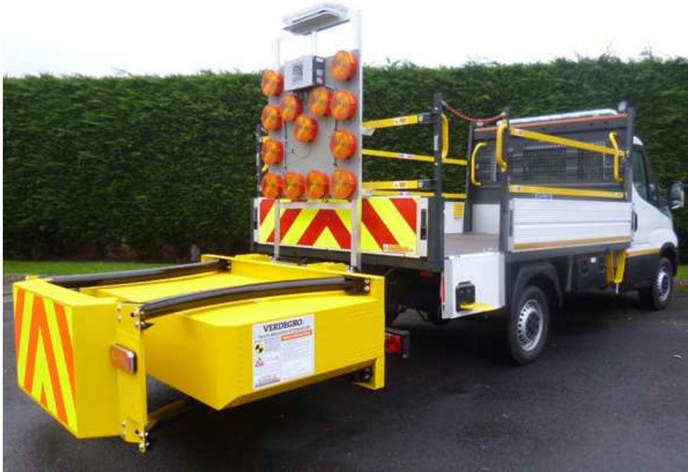
Figure 29. TMA, equipped with crash cushion and various LEDs (beacon bars, work lights, strobes). Source: www.roadsafety.co.uk
