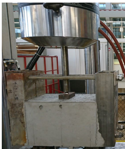
Figure 5. Picture of a tri-axial bending test to form a crack in the notched concrete beam.
