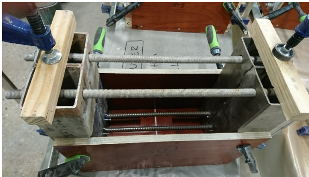
Figure 3. Top view of the formwork used to pour the concrete beams.
