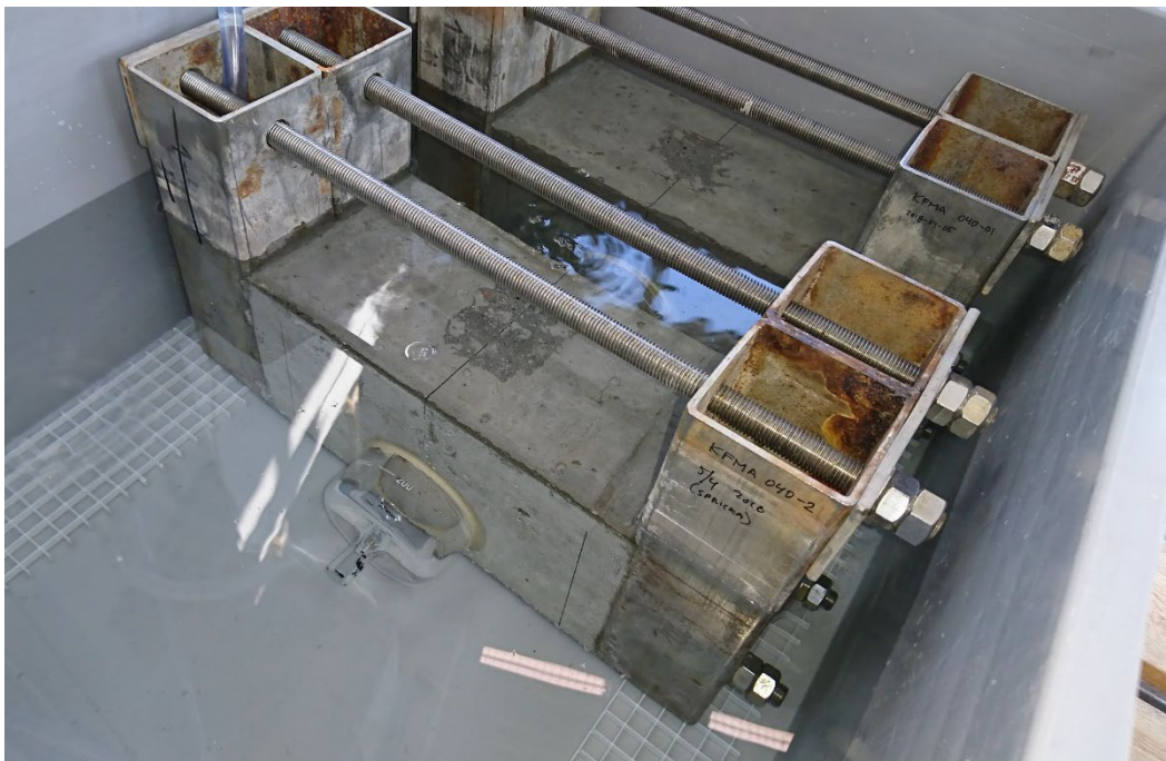
Figure 10. Two cracked beams stored submerged in (de-ionized) water in a large polymer container.
