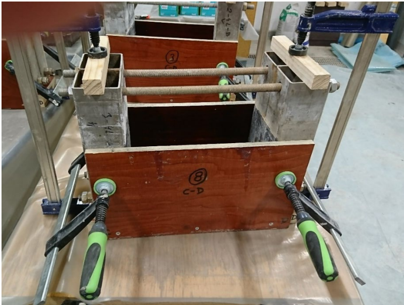
Figure 2. The formwork for the concrete beams.
