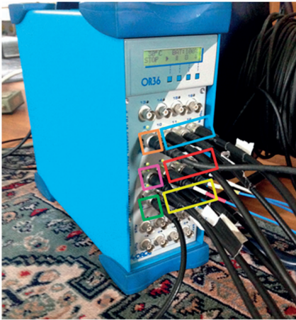
Figure 6-1, standard setup for 12-channel vibration measurement. Photo and text by Teresa Fernández Espejo
