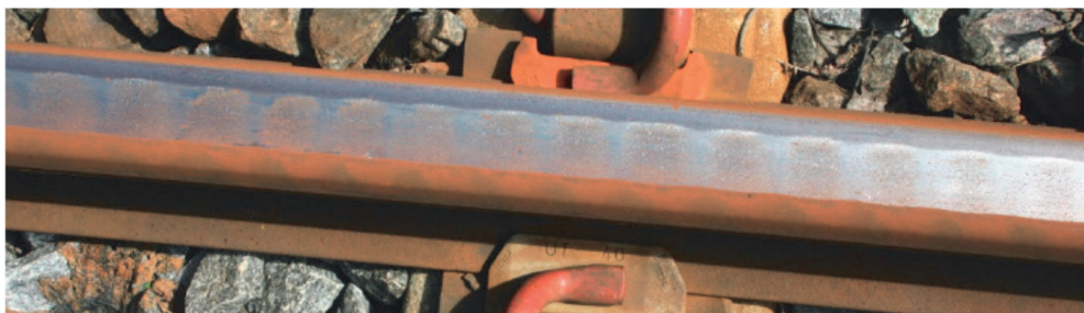
Figure 2-4, example of a rail after many years of wear by one type of metro train at nearly the same speed
