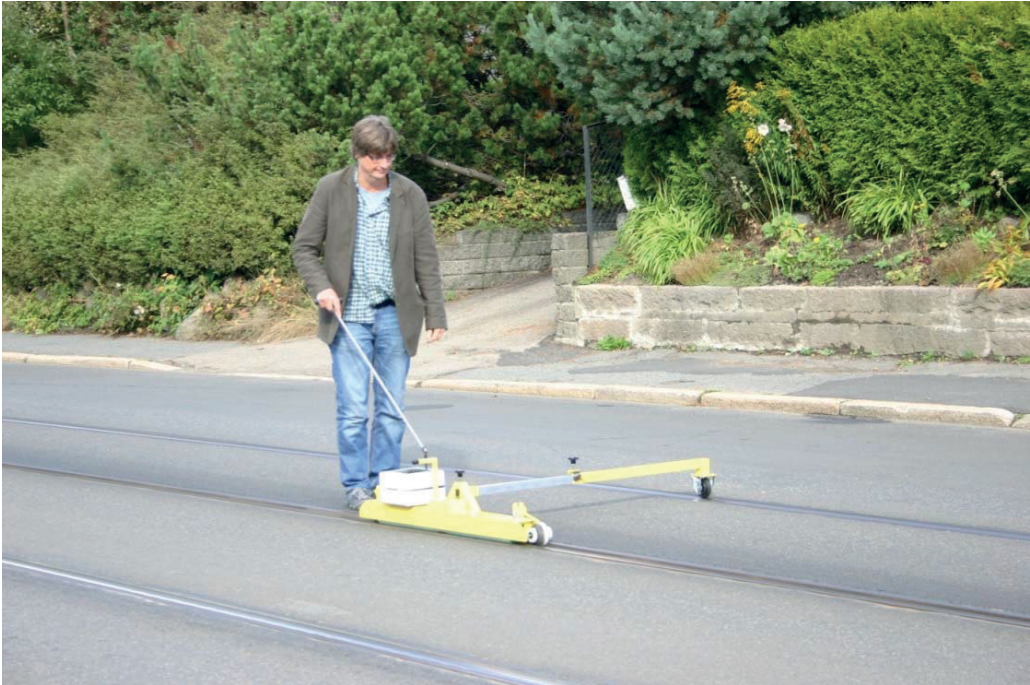
Figure 2, example of rail corrugation measurement
