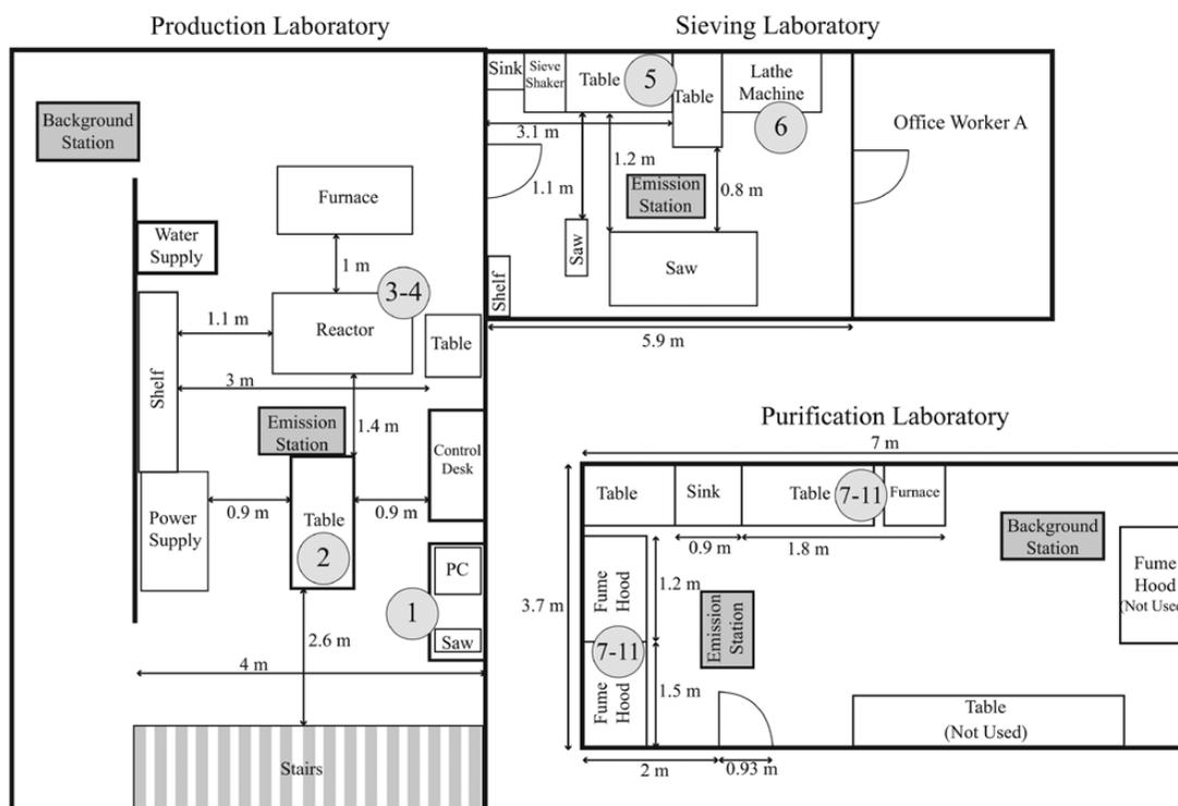
Figure 1 Schematic layout of the facility. Numbers in grey circles correspond to work tasks in Table 1. The production and sieving laboratories were located on a different floor from the purification laboratory.
