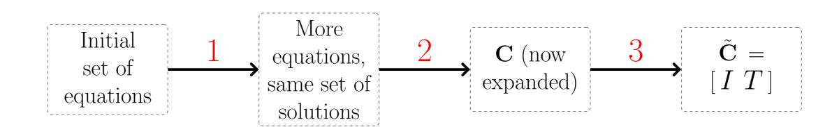
1. Multiply with a set of monomials, 2. Stack coefficients in a matrix, 3. Put C on reduced row echelon form (elimination step).
