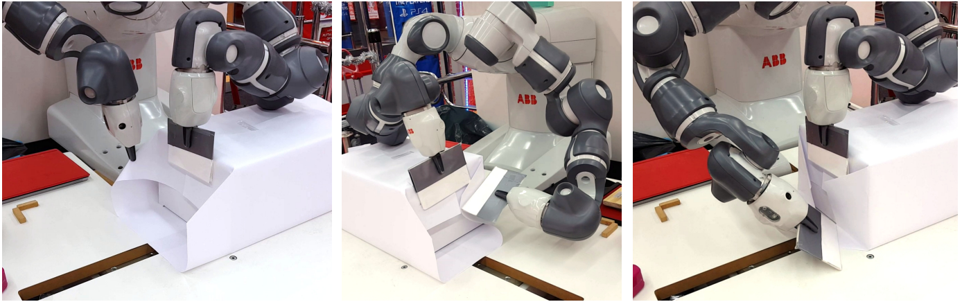
Fig. 6. Folding of the short side flaps. Left: One arms holds down the paper on the short side using the spatula while the other arm uses the fingers to pinch the paper to fold the side flaps. Center and right: The spatula was used to fold the short side flaps by swiping over the paper.
