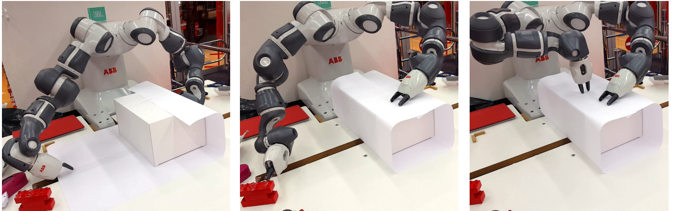
Fig. 4. The folding of the long side. Left: The incision in the table top was used to pick up the paper. The left arm fixates the package by holding from the side. Center: The right arm has put the paper on the package and handed over to the left arm to hold it, while the right arm fetches a piece of tape. Right: The right arm attaches the piece of tape to the package.
