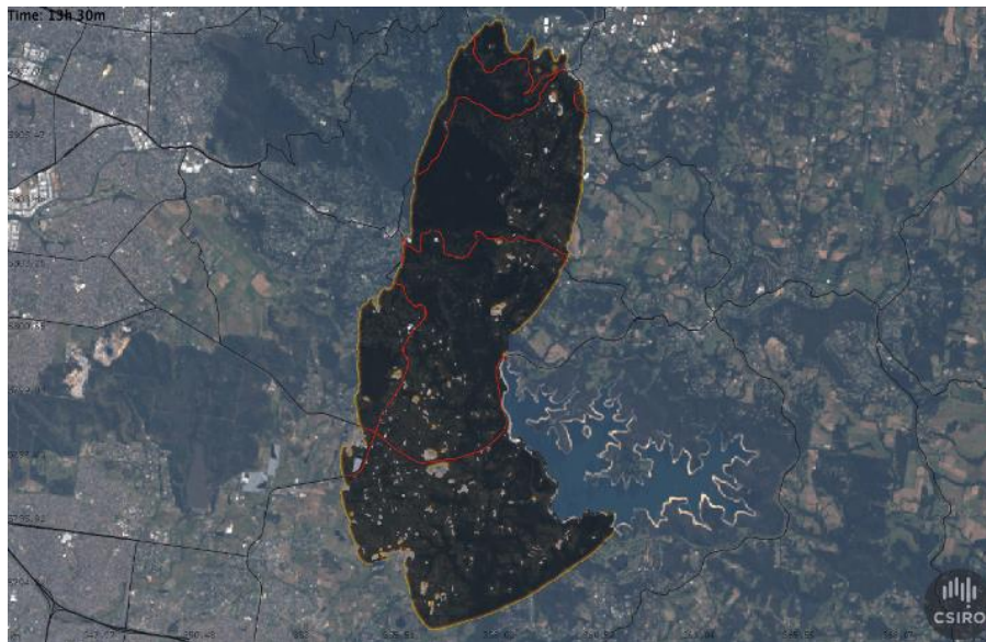
Figure 41. An output of Spark fire model showcasing a fire perimeter on Australian vegetation highlighting the area threatened from a particular fire. 104
