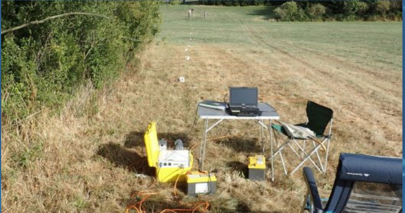
Figure 2. Geophysical SIP field measurement along a profile at a test site in Germany
