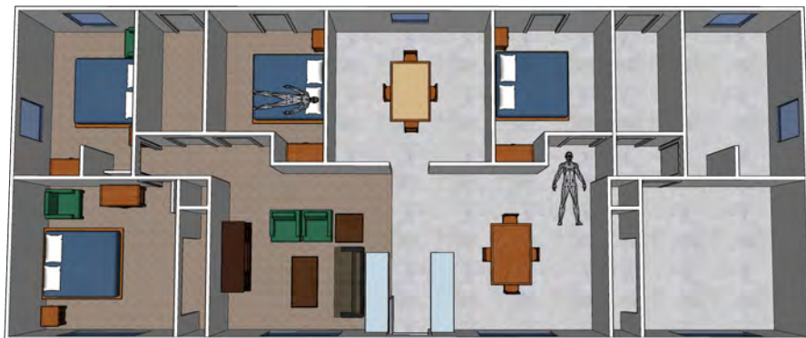
Figure 5.7: Layout of burn structure and location of occupants.
