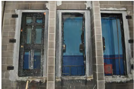
Figure 23. Door samples after the test.
