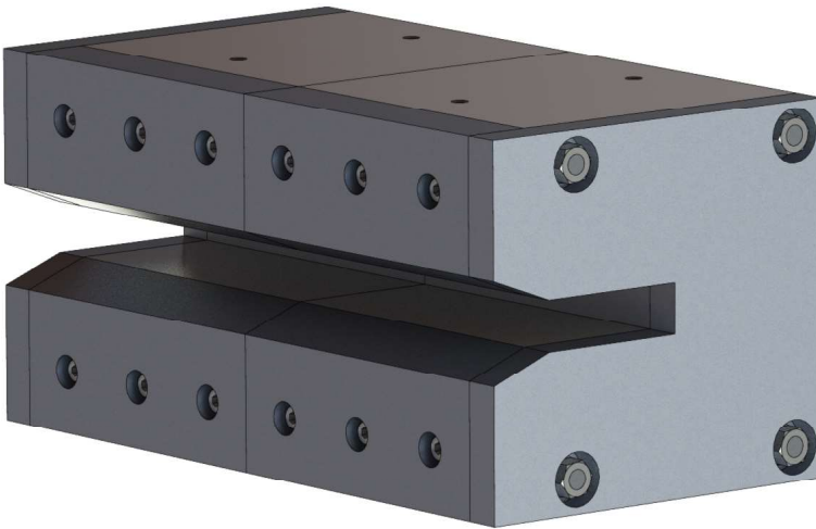
Figure 4.2: Spectrometer dipole magnet render. Rendered CAD model image of the electron spectrometer dipole magnet designed and used for LWFA experiments at the Lund High-Power Laser Facility. The nearest outermost surfaces are aluminium spacers. The shinier magnet blocks are visible inside the gap, and the internal wall is also an aluminium spacer.
