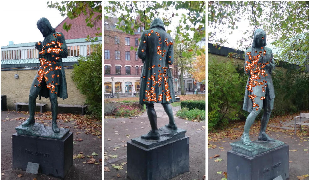
Figure 2.13: The figure shows three frames of the Linnaeus sequence. Also shown are the tracked Harris points (orange circles) and the reprojected points (white dots) using the proposed method. For visibility a random subset of 250 points are shown
