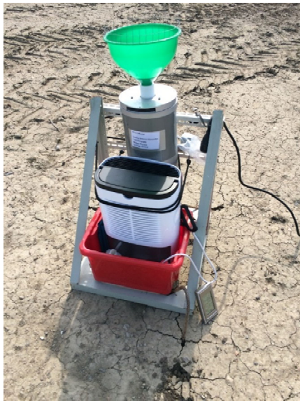
Figure 4: The air humidity sampler Wood's MRD10 located in front of the Palmex rain sampler.
