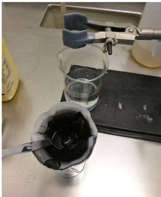
Figure 2: Example of filtration setup
