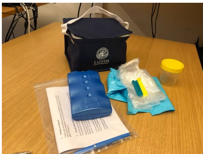
Figure 21: Sampling kit including a sample bottle, a cooling bag and a questionnaire to fill in.
