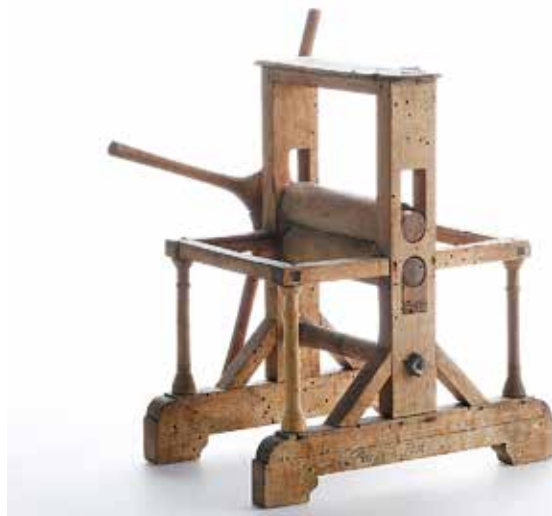
Fig. 4.11. Wooden model for a plate printing press made by Johan Leche in 1738. Fysicum 402. Photo: Gunnar Menander.
