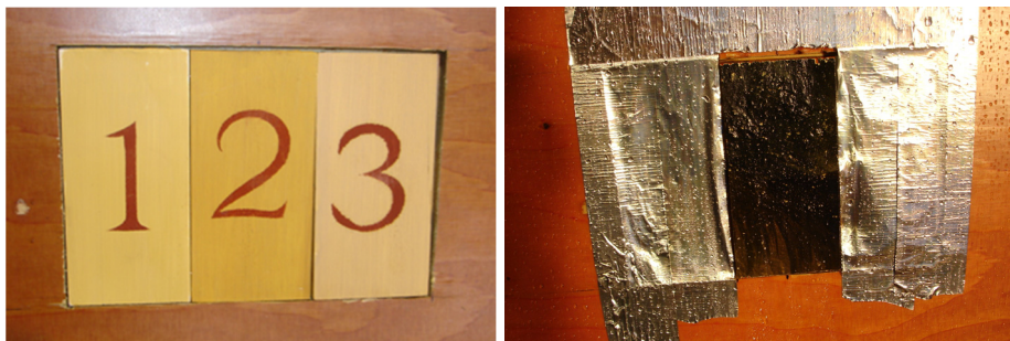
Figure 16 The newly made (left) and authentic test samples when installed at the wall. Photos: Magnus Arvidson.
