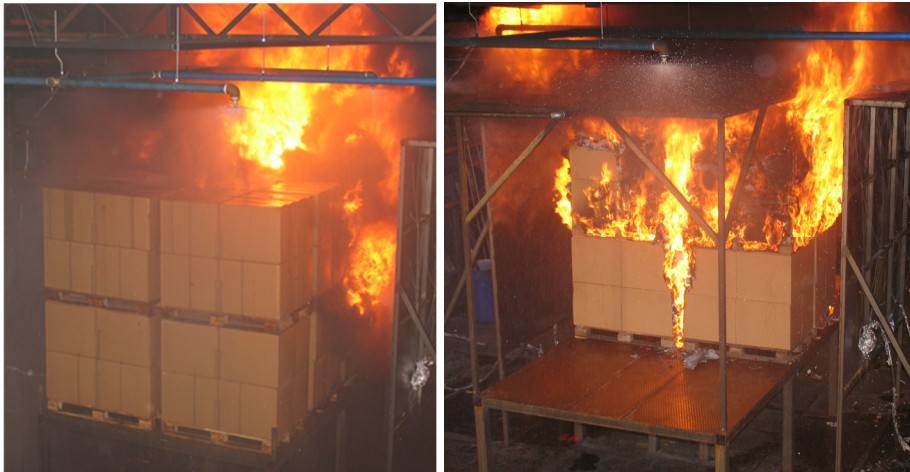
Figure 10. An illustration of the arrangement of the commodity on the trailer mock-up with and without the roof. Steel sheet screens instrumented with thermocouples were positioned on either of the long sides. Note that less amount of commodity was used for the latter tests. Photos: Magnus Arvidson.
