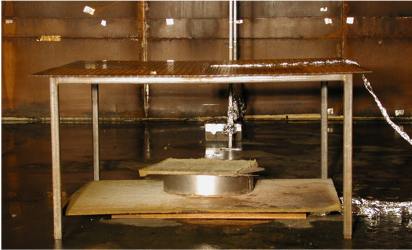
Figure 6 One of the pool fire trays when positioned on the load cell under the obstruction steel plate. Photo: Magnus Arvidson.
