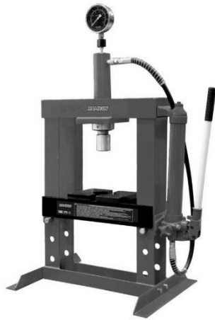
Fig. 1. The hydraulic hand-press for producing the NaCl pellets. A special made tool (Fig. 2) was developed for this press.
