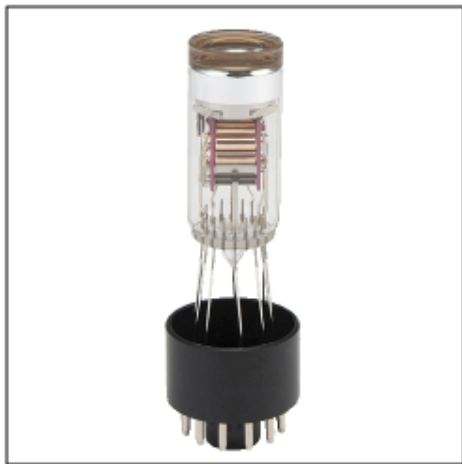
Figure 3. Images of photomultipliers used in PET.
