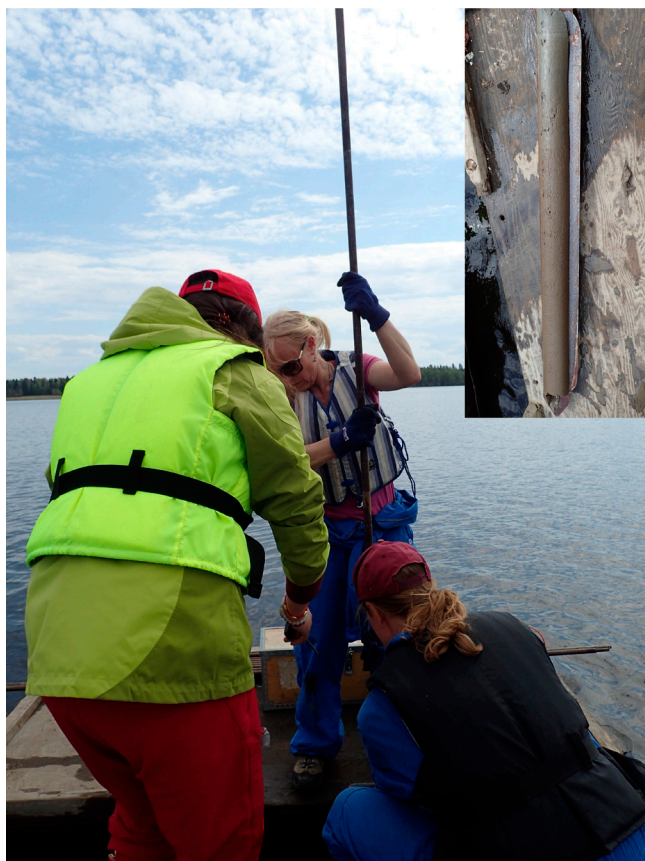
Figure 4 Sediment sampling in Lake Stora Hästefjorden and a sediment core retrieved by a Russian corer.
