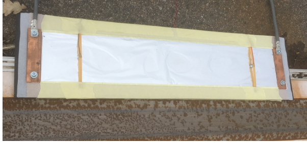
Figure 3.10: The experimental board for measuring the cooling effects by vehicles, figure from [74].
