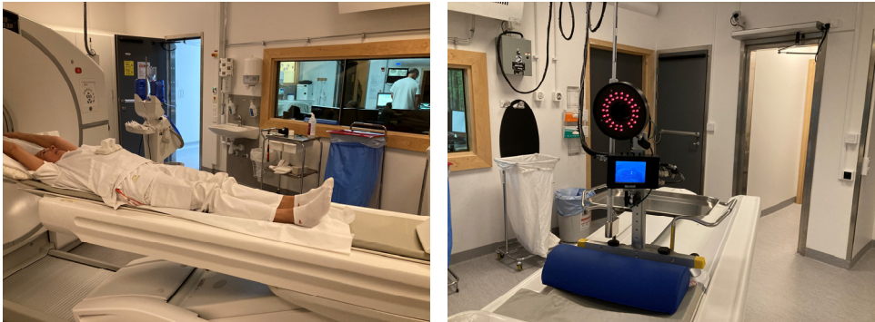
Figure 6 Infrared camera mounted on the PET/CT table and an infrared reflective marker block that is fixed to the patient chest.
