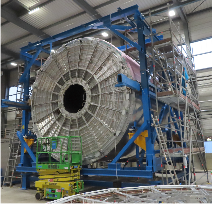
Figure 4.6 – Photograph of the TPC, when it had been taken out from the ALICE cavern for the upgrade. At this stage, the old readout chambers had been removed and the TPC was about to be moved to a cleanroom for installation of the new ones, so only the field cage (and the wire chambers, which were not yet removed) remained.
