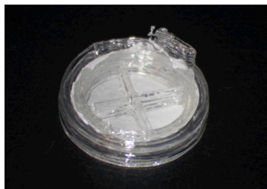
Fig. 1. Image of the 3D fibre unit consisting of the uncompressed PCL fibre mesh supported in lock-rings made of PLA. The fibre mesh that is very delicate is kept from bulging by a cross-shaped structure made of PLA. The diameter of the set-up is 10 mm and it is placed in a well of a hydrophobic 48-well plate before seeding of cells.
