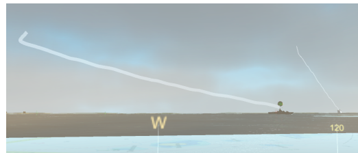
Figure 11: The bright bearing-lines in the sky indicates that both visual ships are steering to the right. The ship to the right is farther away, which is visualized with the thinner line. The ship to the left is going at a constant speed but has made a turn approximately 25 seconds ago. 30 seconds of history is presented in the CEP.
