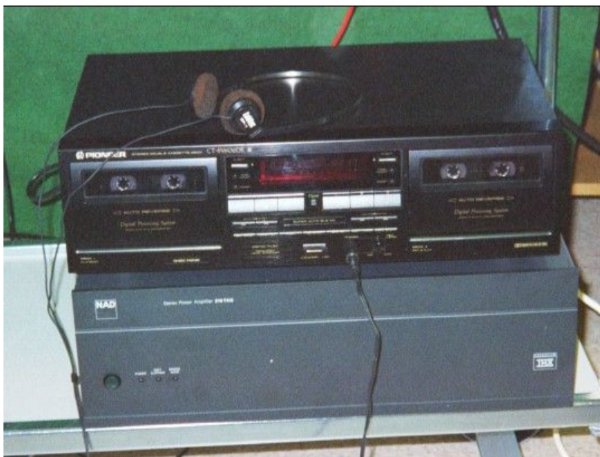
Figure 3 Cassette recorder with output signal connected to a sound power amplifier. The Helmholtz coils are connected to the amplifier's speaker output. The signal cassettes were obtained from Litovitz.
