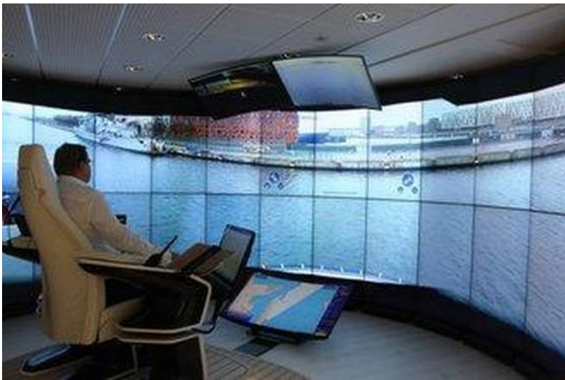
Figure 2.7: A GUI used for teleoperation of a tug in Copenhagen. Image from Kongsberg Maritime [54]. Used with permission.
