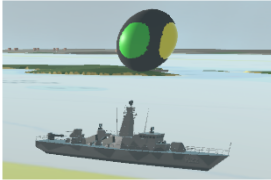
Figure III.10: From the AIS data, the ship type, position and heading is extracted. From the ship type, a suitable 3D-model is chosen. The sphere is positioned above the position, and is colored according to the heading.
