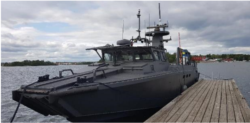
Figure 2.6: The patrol boat, rebuilt from a Combat Boat 90H.
