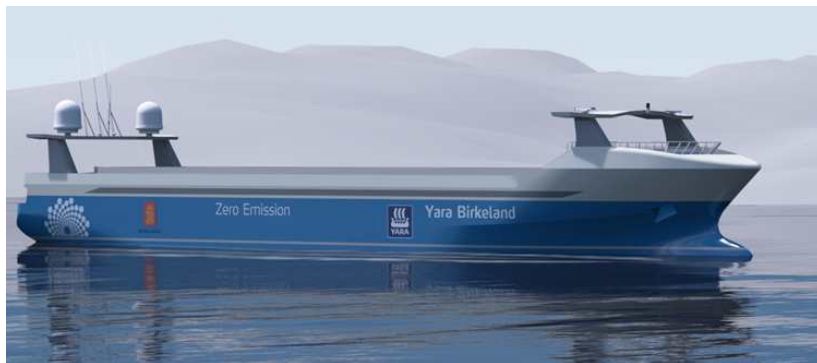
Figure 2.2: A battery container ship named Yara Birkeland, constructed to be fully autonomous. Image from Kongsberg Maritime [54]. Used with permission.
