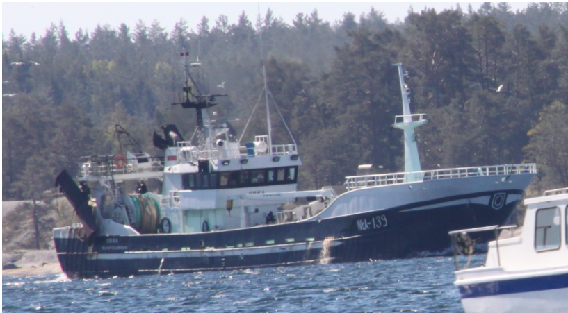
Figure 1.1: GT is a measurement unit of volume, and 260GTs is equal to about 1,000m^3 [8]. As an example, the trawler ORKA, seen in the image, has the volume 468GT.
