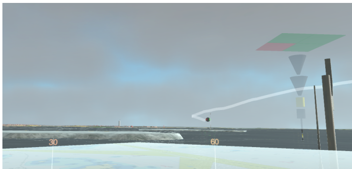
Figure III.9: The South Cardinal Mark marks the grounding north from the Cardinal Mark (to the left in the image). The grounding is also marked with an iceberg.
