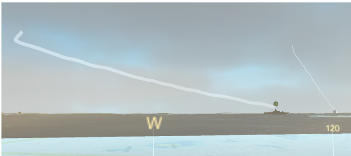
Figure III.11: The bright bearing-lines in the sky indicates that both visual ships are steering to the right. The ship to the right is farther away, which is visualized with the thinner line. The ship to the left is going at a constant speed but has made a turn approximately 25 seconds ago. 30 seconds of history is presented in the CEP.
