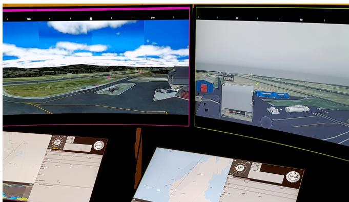
Figure 4.1: A control station of Saab's Remote air traffic control systems . In the figure, two simulated airports are traffic controlled simultaneously by a single operator.
