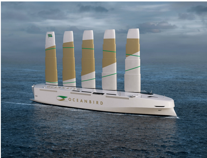
Figure 1.3: The wind-powered sailing ship developed by Wallenius Marine. Image from Wallenius Marine [27]. Used with permission.
