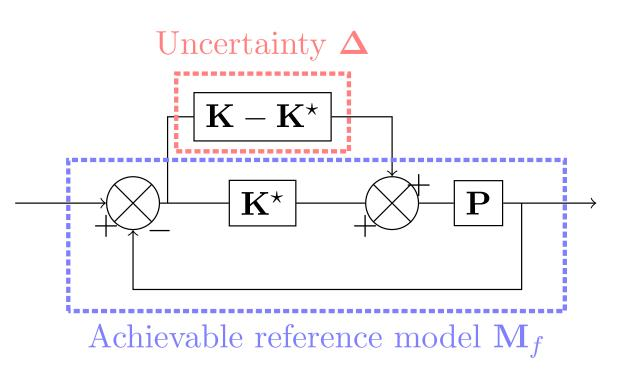
The resulting closed-loop is well-posed and internally stable for all stable  $\Delta$  such that  $\|\Delta\|_{\infty} \leq \beta$  if and only if  $\|(1 - \mathbf{M}_f)\mathbf{P}\|_{\infty} < \frac{1}{\beta}$ .
