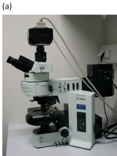
Figure 2.1.1 (a) Picture of PL microscope. (image source: https://en.wikipedia.org/wiki/Fluorescence_microscope ). (b) Scheme figure of luminescence microscope
