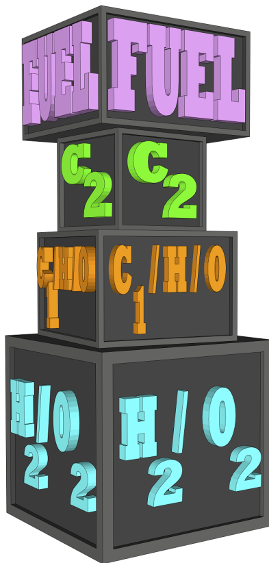
Figure 5.1: Schematic image of the block structure modelling methodology. The methodology is used to create reduced ethylene-air [43], propane-air [11], kerosene-air [20,41,42] and Jet Propellant 10-air (JP-10-air) [81] reaction mechanisms.
