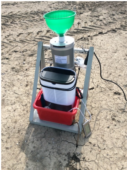
Figure 7 The air humidity sampler Wood’s MRD10 located in front of the Palmex rain sampler.
