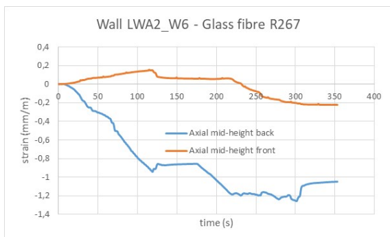
Figure LWA2_W6_3 Axial strains at mid-height vs. time – front (tension) and back (compression) side.
