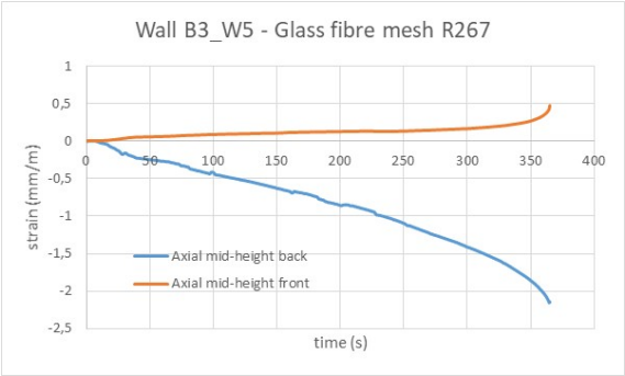
Figure B3_W5_2 Axial strains at mid-height vs. time – front (tension) and back (compression) side.
