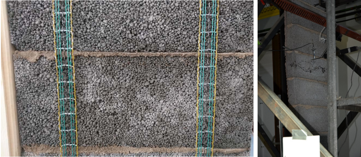
Figure LWA2_W5_1 High strength steel wire strips attached directly to the wall (left); Compression failure at mid-height of the wall (right).
