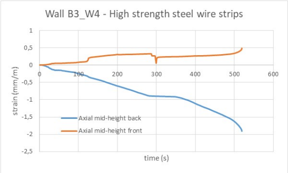
Figure B3_W4_2 Axial strains at mid-height vs. time – front (tension) and back (compression) side.
