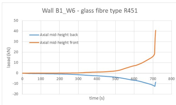
Figure B1_W6_2 Axial strains at mid-height vs. time – front (tension) and back (compression) side.
