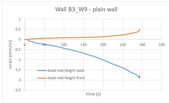
Figure B3_W9_2 Axial strains at mid-height vs. time – front (tension) and back (compression) side.
