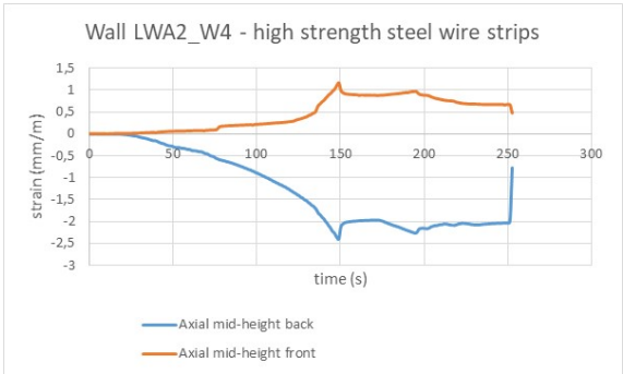
Figure LWA2_W4_3 Axial strains at mid-height vs. time – front (tension) and back (compression) side.
