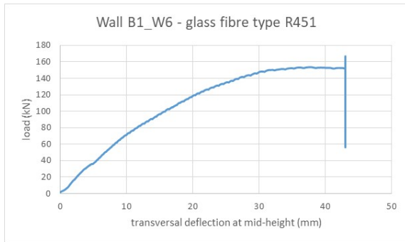
Figure B1_W6_1 Load vs. transversal deflection at mid-height (left); Load vs. time (right)
