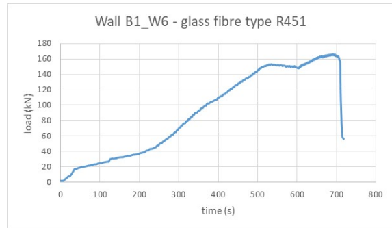
Figure B1_W6_1 Load vs. transversal deflection at mid-height (left); Load vs. time (right)
