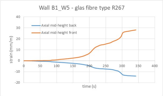
Figure B1_W5_2 Axial strains at mid-height vs. time – front (tension) and back (compression) side.
