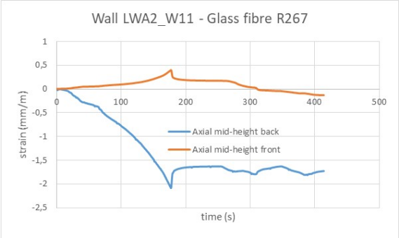
Figure LWA2_W11_3 Axial strains at mid-height vs. time – front (tension) and back (compression) side.
