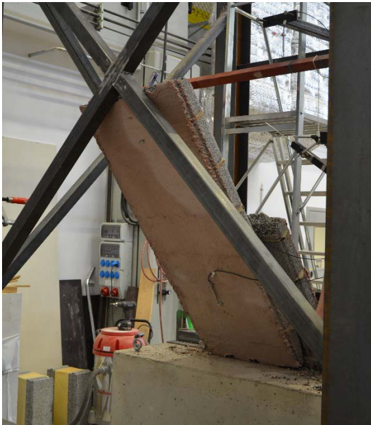
Figure LWA2_W9_1 Flexural tensile failure of the reinforcement at 2/3-height of the wall.
