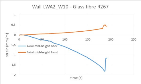
Figure LWA2_W10_3 Axial strains at mid-height vs. time – front (tension) and back (compression) side.
