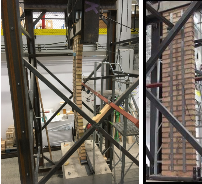
Figure B1_W3_1 Testing of brick wall strengthened with mechanically fastened steel strips.
