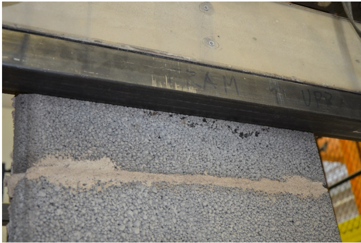
Figure LWA2_W8_1 Local crushing at the upper loading plate.
