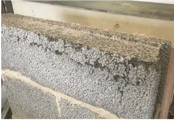
Figure LWA2_W12_1 Local crushing at the upper loading plate.
