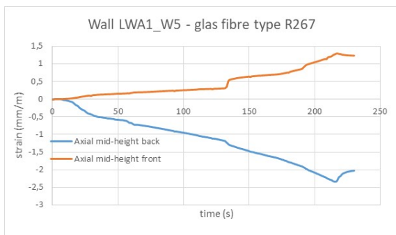
Figure LWA1_W5_3 Axial strains at mid-height vs. time – front (tension) and back (compression) side.
