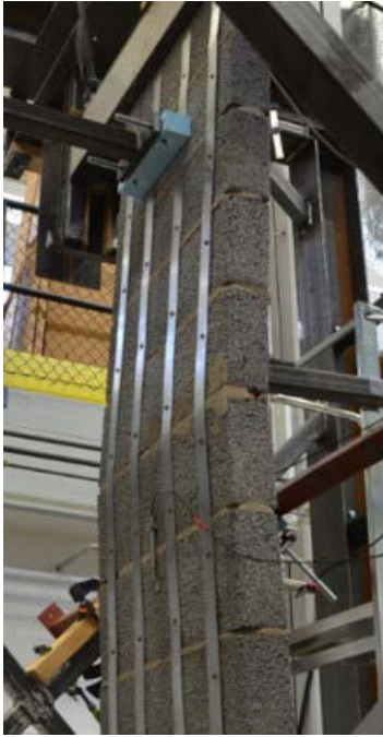
Figure LWA1_W3_1 Mechanically fastened steel strips.
