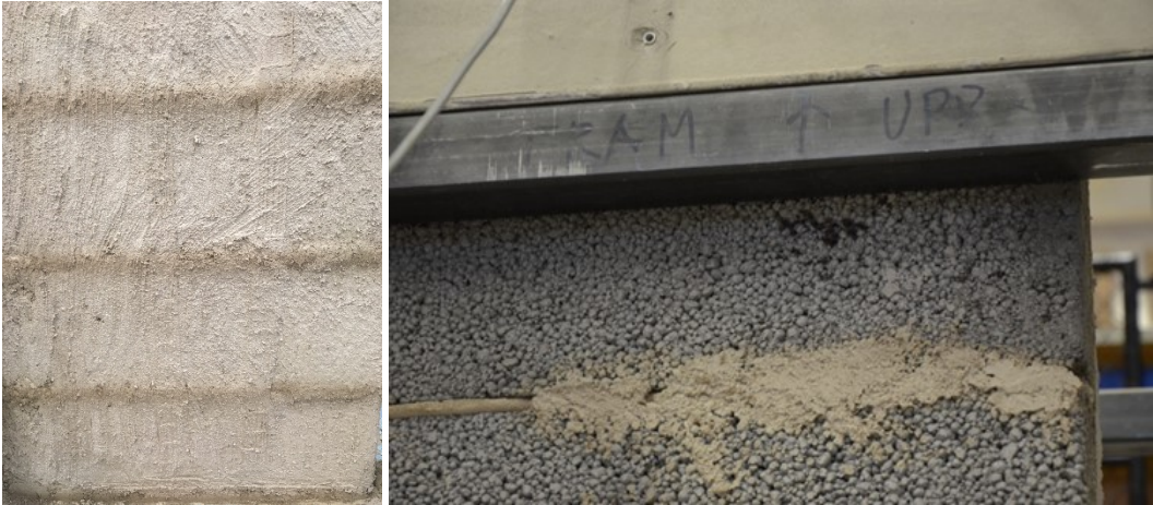
Figure LWA1_W4_1 High strength steel strips (left); Crushing at the load application plate (right).
