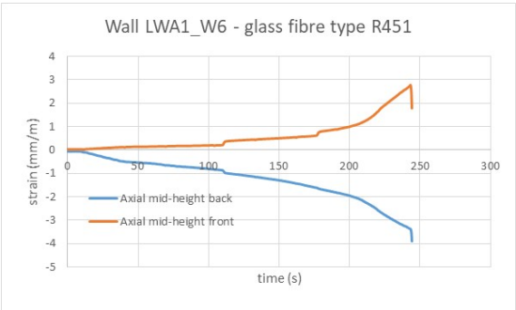
Figure LWA1_W6_3 Axial strains at mid-height vs. time – front (tension) and back (compression) side.
