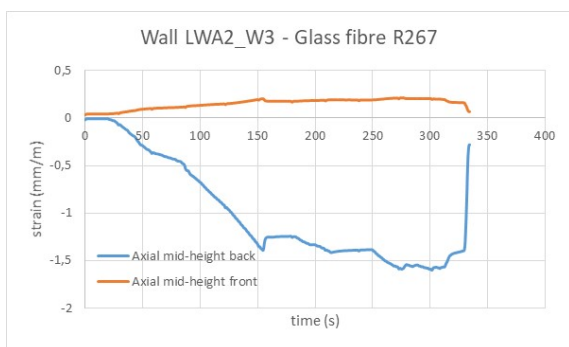
Figure LWA2_W3_3 Axial strains at mid-height vs. time – front (tension) and back (compression) side.
