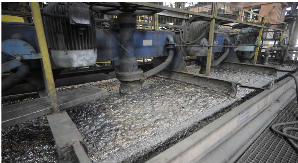
Figure 1.3 Flotation process to obtain metal concentrate.
