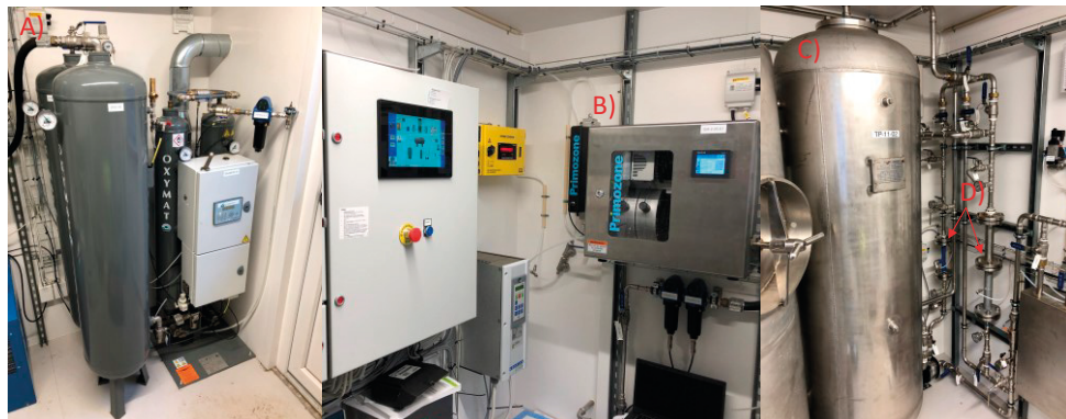
Figure 3. Three photographs of the machine room of the ozone pilot plant. A) pressure swing adsorption module and oxygen tank, B) ozone generator, C) reaction tanks and D) Venturi injector (left) and static mixer (right).
