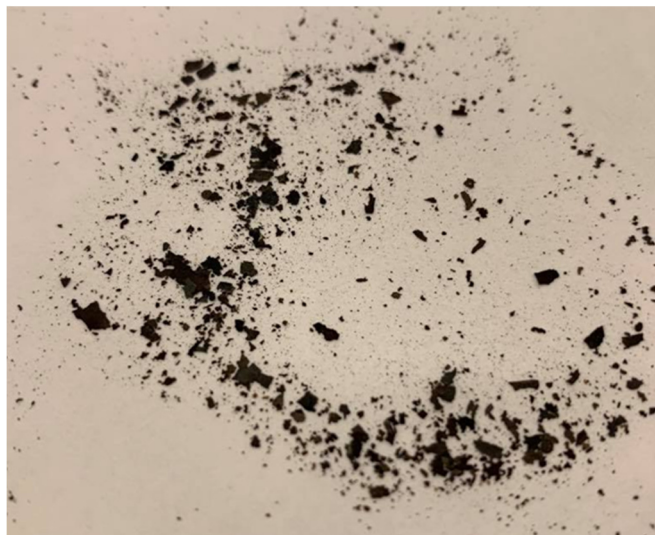
Figure 3.6. The coke formed in the CFR system after Indulin AT depolymerization at 250 °C.
