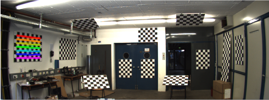
Figure 2.2: Calibration setup for one of the sequences in the famous KITTI dataset, where OpenCV’s findChessboardCorners has been used to find the leftmost chequerboard. The radial distortion is noticeable on the sides of the image, where physically straight lines appear to be curved. This phenomenon is not compatible with the pinhole camera model, and thus must be compensated for prior to estimating the relative pose between images. Image credit: KITTI dataset [23].
