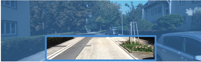
Figure 8: Image from the KITTI Visual Odometry / SLAM benchmark, Sequence 03. The cropped area (contained within the thick border) depict the image used to compute the homographies. Image credit: KITTI dataset [4].
