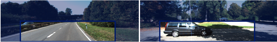
Figure 5: Images from the KITTI Visual Odometry / SLAM benchmark, Sequence 01 (left) and 03 (right). Since the algorithm is homography-based the images are cropped a priori in order to contain a significant portion of planar or near planar surface. Such an assumption is not valid on all sequences of the dataset, however, certain cases, such as the highway of Sequence 01 (left) is a good candidate. There are several examples where occlusions occur, such as the car in Sequence 03 (right). These situations typically occur at crossroads and turns. Image credit: KITTI dataset [9].
