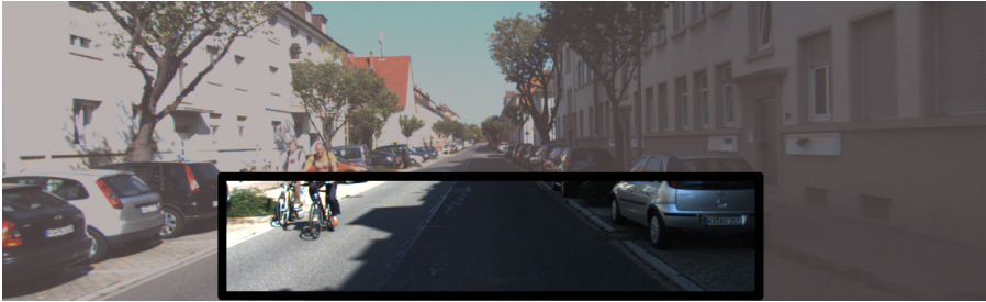
Figure 6: Image from the KITTI Visual Odometry / SLAM benchmark, Sequence 00. The thick black border indicates the area which is cropped prior to estimating the homography. This is only a crude approximation, and cannot guarantee that the image only depicts a planar surface, which is clearly shown as the bicyclists pass by the car, as well as the vehicle parked to the right. This, however, shows that the proposed method is robust enough to deal with violations of the planar motion model. Image credit: KITTI dataset [2].
