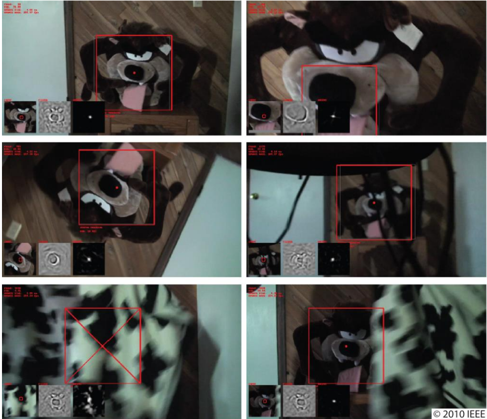
Fig 5.1. Example of a correlation filter based adaptive tracker (MOSSE) that is able to keep track of the target despite zooming in and re-locate the target after an occlusion. The miniature pictures respectively display the input from the estimated target position, correlation filter, and the result of convolving the correlation filter over the image (estimated new position). Figure taken from Bolme et al. (2013).
