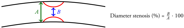
Figure 1.11: Illustration of how the diameter stenosis is determined using QCA, by measuring the minimal lumen diameter B compared with the reference diameter A .
