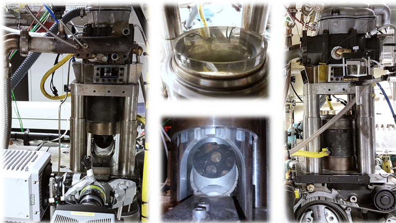
Figure 3.3. Images from an optical engine converted according to the Bowditch design. In this case, drop-down liner is used, a flat-top piston and three liner windows are used to obtain lateral access inside the combustion chamber
