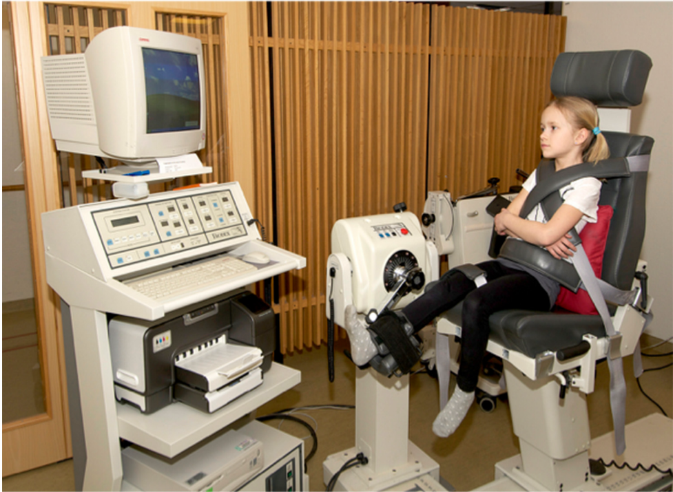
Figure 19: A child participating in the POP study being assessed in a Biodex computerized dynamometer
