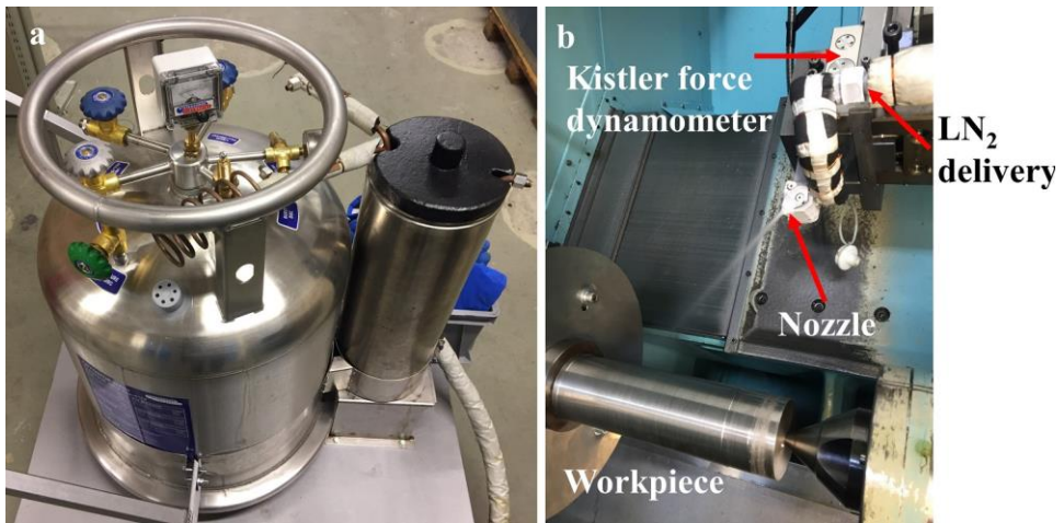
Figure 3.3. (a) Cryogenic distribution system; (b) Cryogenic machining setup.
