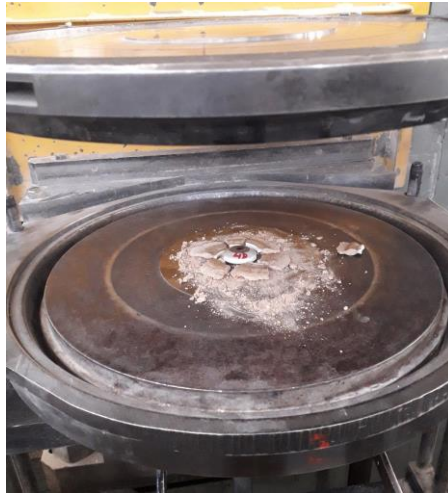
Figure 3.2. Toroidal high-pressure cell used for HP-HT treatment of the diffusion couple sample.
