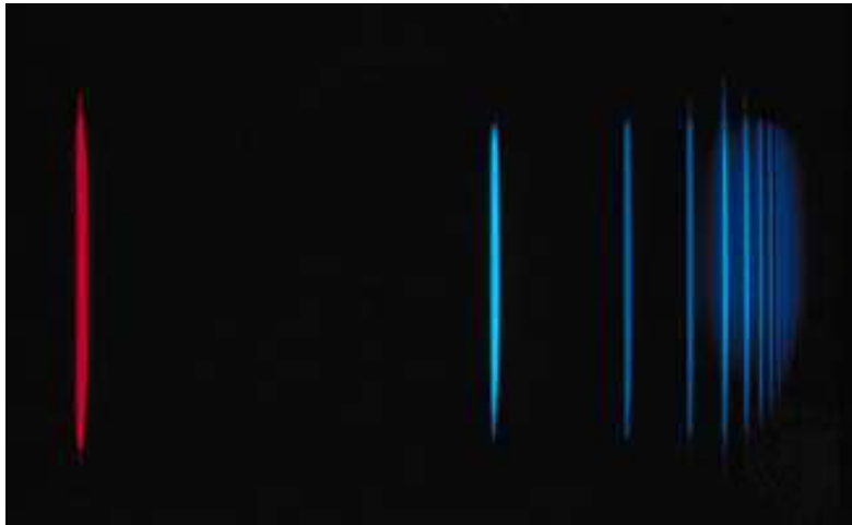
Figure 2.1: Portion of the hydrogen spectrum observed by a low-resolution spectrometer corresponding to the Balmer series. https://www.britannica.com/science/spectroscopy/Basic-properties-of-atoms
