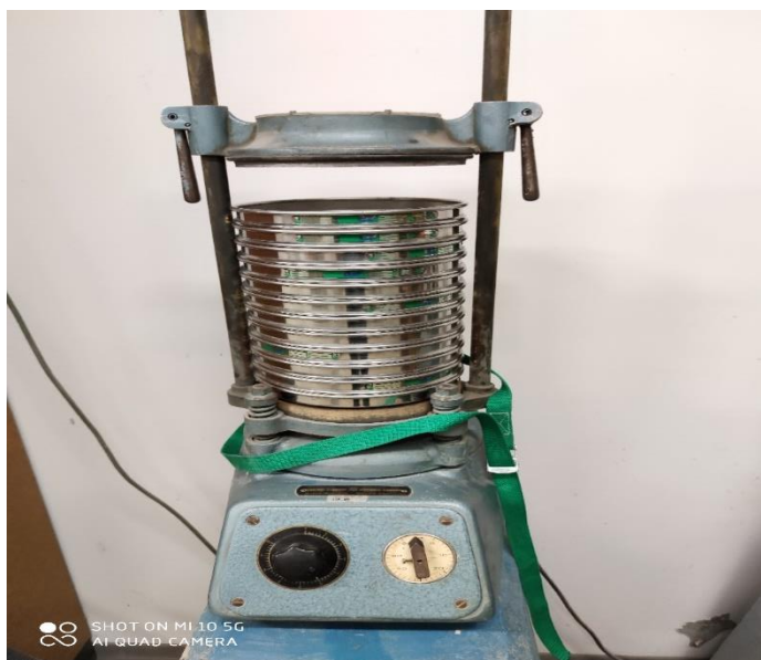
Figure 10. Sieve set with sieve shaker
