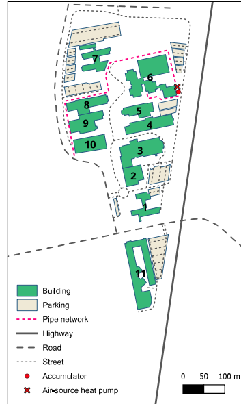
Fig. 2. Map of the eleven buildings included in the case study. The map was created using QGIS program for the analysis of geospatial data.
