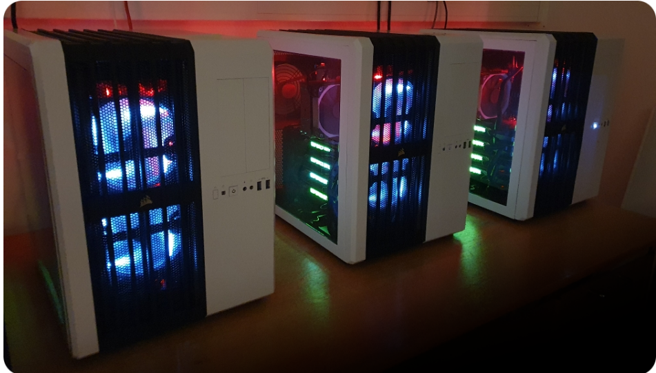
Figure 1.4: Picture of the server specifically designed and constructed for the Monte Carlo simulation of photon transport using Multi-Scattering . It consists of 3 computers each containing 4 Nvidia GeForce GTX 1080Ti cards.
