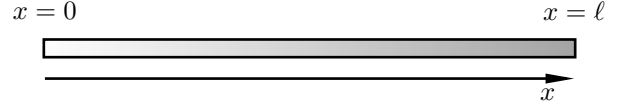
Figure 1: Rod of length \ell with one-dimensional spatial coordinate x and conductivity k(x) = x^2 + 1 .
