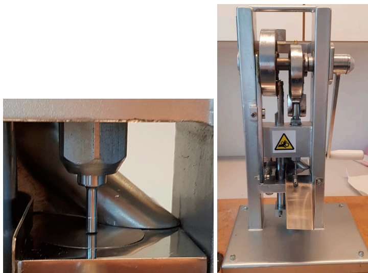
Figure 6. The standard desktop tablet press tool used for making the pellets in Paper IV (right). The left image shows a close-up view of the die cavity and the upper punch.
