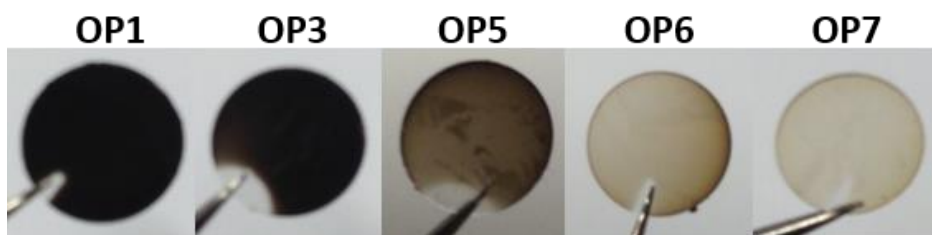
Figure 2.6. Sampled mini-CAST soot on a small sapphire glass. As can be seen, the colour appears different of the various soot types as the OP1 and OP3 soot is black, while the sampled OP5-7 soot gives a more brownish and yellow colour. Note that the collected mass varies between the samples and may hence influence the true relative colour. With courtesy of Thi Kim Cuong.
