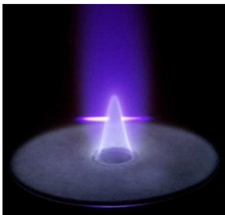
FIG. 1. Photo of a premixed methane/air flame ( \phi = 1.0 ) seeded with 10 ppm TMI. A narrow 410 nm laser beam sent horizontally from left to right through the flame is manifested by laser-induced fluorescence from indium atoms.
