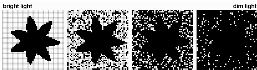
Fig. 2 The effect of photon shot noise.
