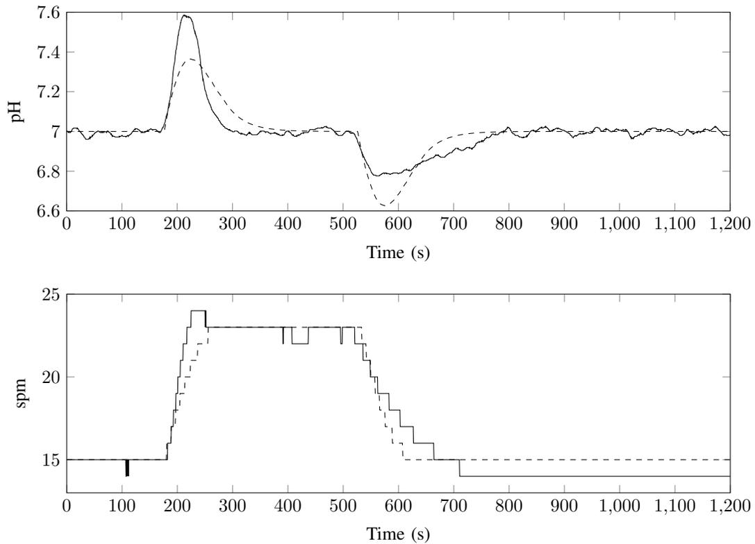
Fig. 4. Closed-loop load disturbance attenuation experiment: plant output (top) and controller output (bottom). Experimental data is shown in solid, simulated in dashed. The disturbance enters at the plant input as a pulse of height  $-8$  being active from the instant 150 to 500.
