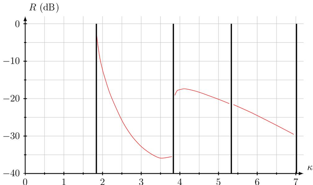
**Figure 6:** The reflected power in a dB-scale in the waveguide as a function of the normalized frequency  $\kappa$ . The vertical lines give the location of the cutoff frequencies in the circular waveguide.
