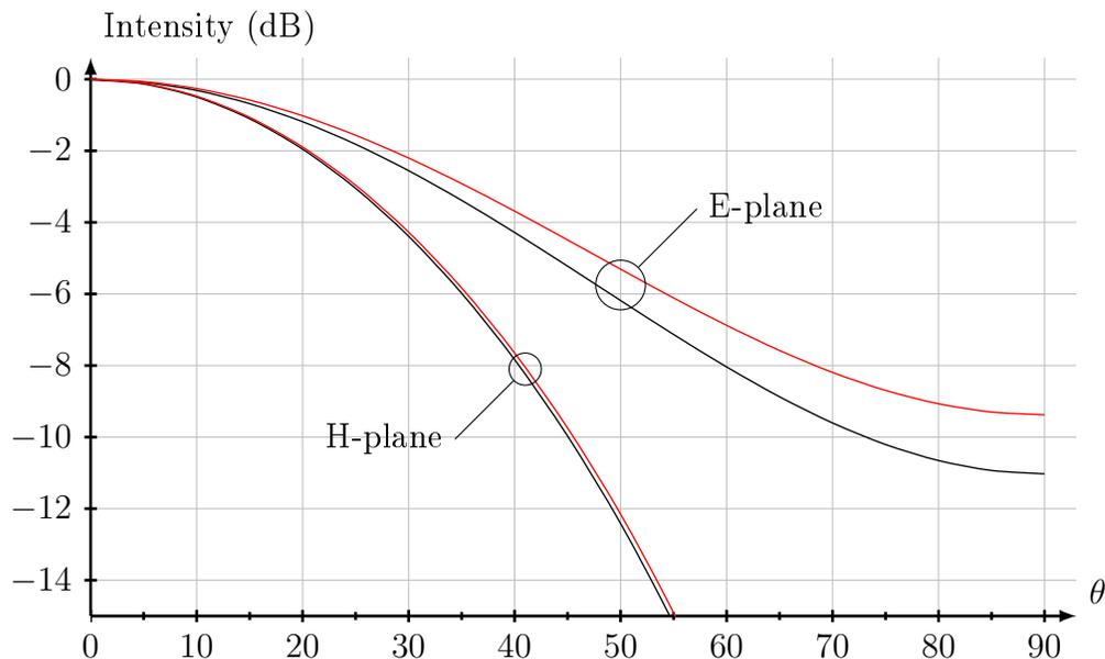
**Figure 4:** The normalized intensity in a dB-scale as a function of the observation angle  $\theta$  at the normalized frequency  $\kappa = k_0a = 1.01\eta_{11} \approx 1.86$  (E-plane and H-plane). The black lines are the exact solutions, while the red lines are the approximate solutions (see text), when the aperture field is identical to the incident mode.
