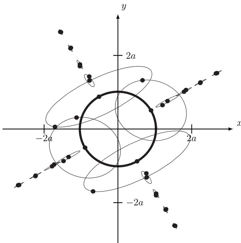
**Figure 7:** The polarization ellipse of the surface current on the ground plane at the normalized frequency  $\kappa = k_0 a = 1.5\xi_{11} \approx 5.75$ . The dots at the center of each ellipse locate the points at which the currents are computed and the dots on the ellipse give the currents at a synchronized time. The thick circle locates the circular aperture  $r_c = a$ .
