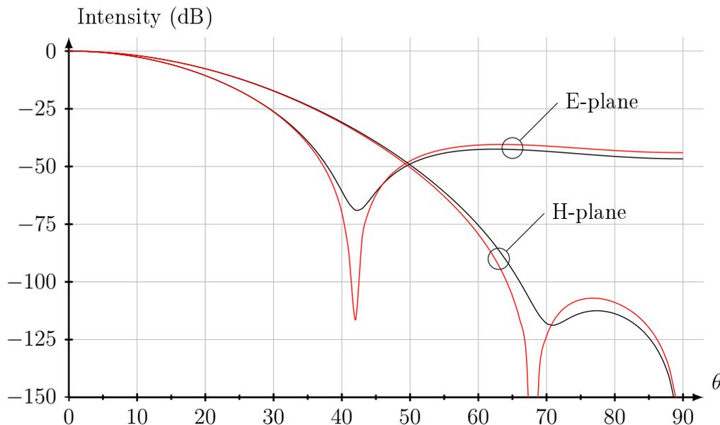
**Figure 5:** The normalized intensity in a dB-scale as a function of the observation angle  $\theta$  at the normalized frequency  $\kappa = k_0 a = 1.5\xi_{11} \approx 5.75$  (E-plane and H-plane). The black lines are the exact solutions, while the red lines are the approximate solutions when the aperture field is identical to the incident mode.
