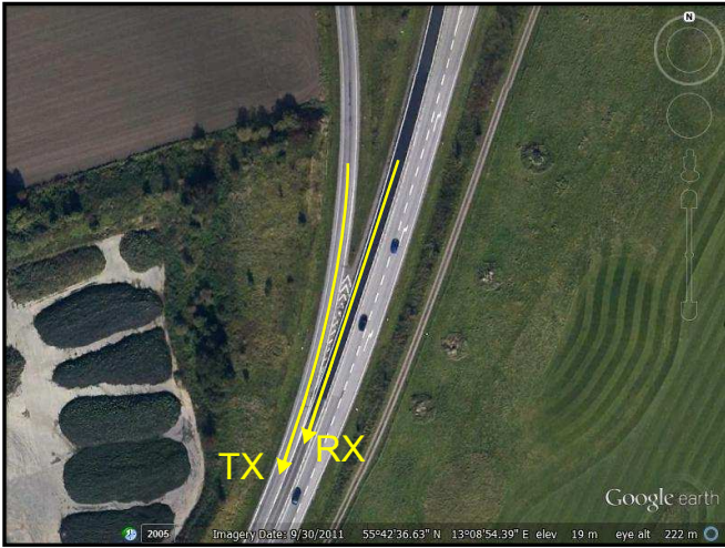
Fig. 1. Google Earth TM [14] aerial image shows the investigated merging lane scenario outside the city of Lund. The TX enters the highway while RX is approaching the merging point on the highway. (N 55°42'36", E 13°8'53")
